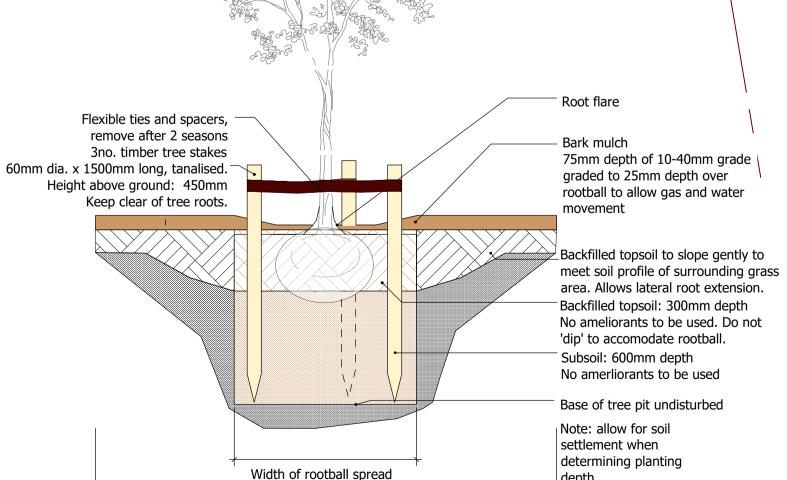
Tree Pit Detail: triple staking
